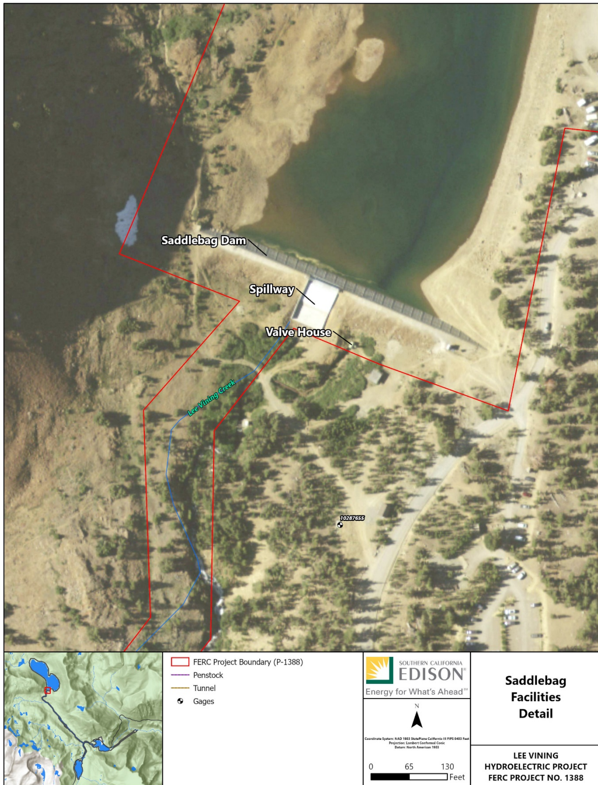
Figure 4.5-1. Saddlebag Lake and Dam Facilities Detail.
