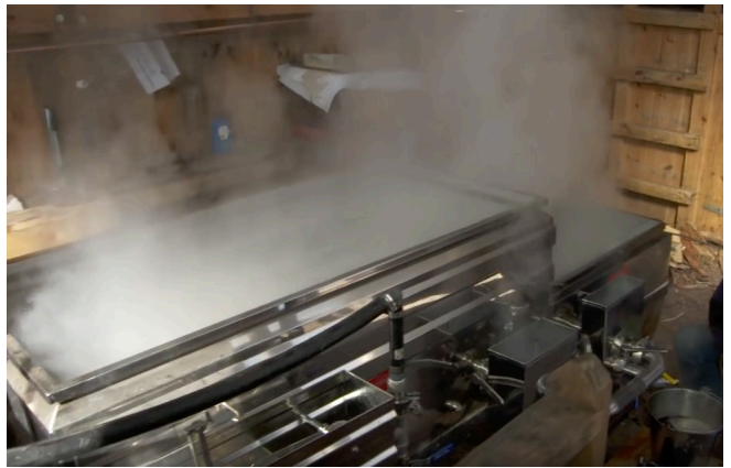
Boil the sap to let the water evaporate and create syrup
