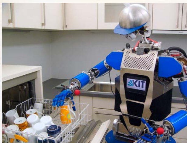
The ARMAR robots developed at the Karlsruhe Institute for Technology (KIT) carry out complex tasks in a kitchen setting, learn from humans and interact with them using natural speech
