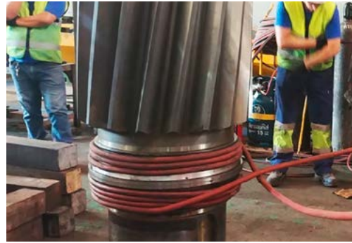
The inner bearing ring is heated on the shaft using an inductor, which facilitates removal
