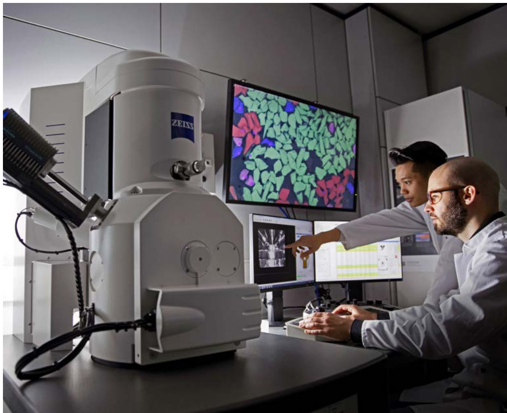
Analytical methods (here: metal analysis using an electron microscope) and capacities will be flexibly adapted to technological change in the future Central Laboratory
