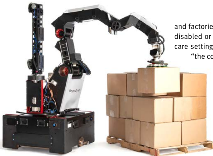
The logistics robot Stretch is expected to be launched in 2022. It can move up to 800 boxes per hour. Its price has not been announced yet
