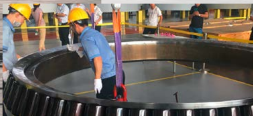
Mounting the taper roller bearing inner ring
