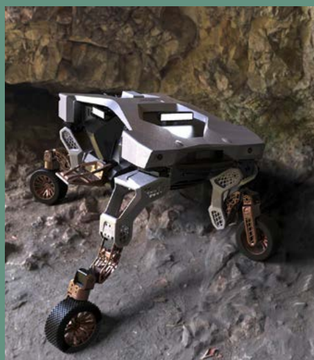
Forward, backward, sideways: the TIGER concept vehicle unites walking and rolling as forms of locomotion, which makes it extremely agile and versatile
