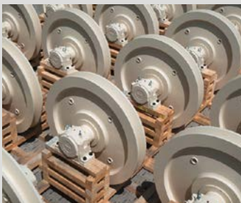
Waiting to be installed: rope sheaves with Schaeffler bearings
