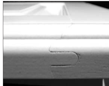
Example of end joint separation
