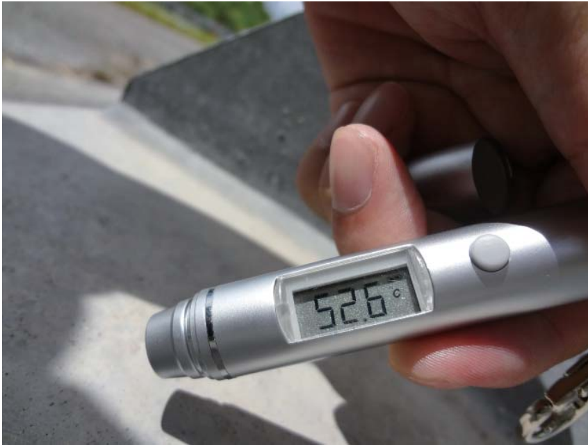
Figure 1. Hot highway guardrail under strong summer solar radiation. The temperature measured on the rail was 52.6°C.
