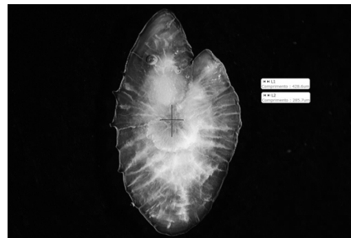
Figure 3. Anchovy otolith with a translucent nuclei and the vertical and horizontal axis for measurements.
