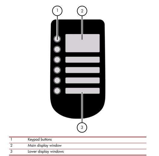
The uPrint SE and uPrint SE Plus display panel and keypad consist of a multiple-line LCD window with two buttons used for scrolling through messages and four single-line windows, each with one button for making selections. The top line in the upper window always shows the printer status.
