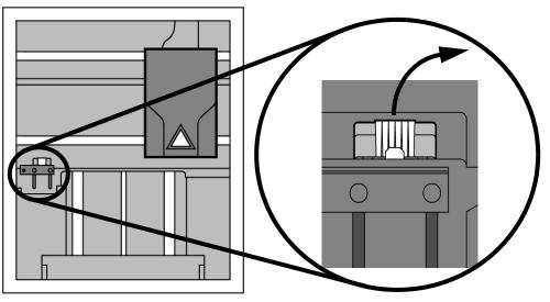
4. Place the new tip wipe assembly over the two mounting posts making sure the assembly is fully installed. See Figure 30.
