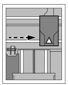
**3.** Remove the tip wipe assembly by lifting the assembly up and out of the printer. Discard this tip wipe assembly. See Figure 29.
