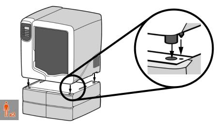
**16.** Remove the black plugs from the model and support Y blocks by pushing in on the coupler rings and pulling outward.
