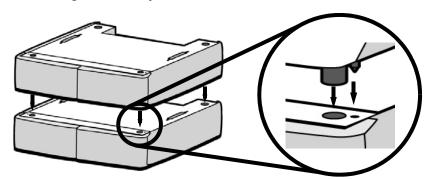
**15.** With 2 people, position the printer on to the top of the material bays. Be sure the feet and pins are properly aligned. See Figure 10.
