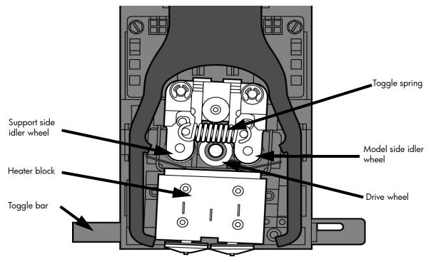
Figure 54 Toggle bar in neutral position
