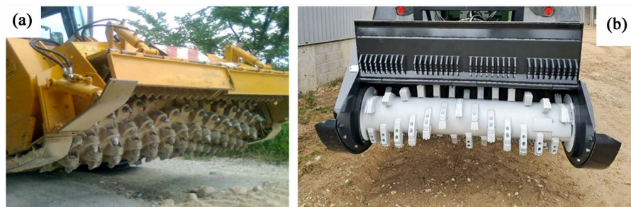
Figure 7. (a) Stone crusher with teeth for calcareous rocks and (b) with hammers for granite rocks.
