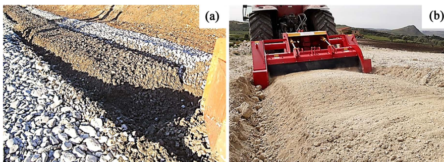
Figure 8. (a) Crushing efficiency on granite rocks; (b) Stone crusher on calcareous rocks.
