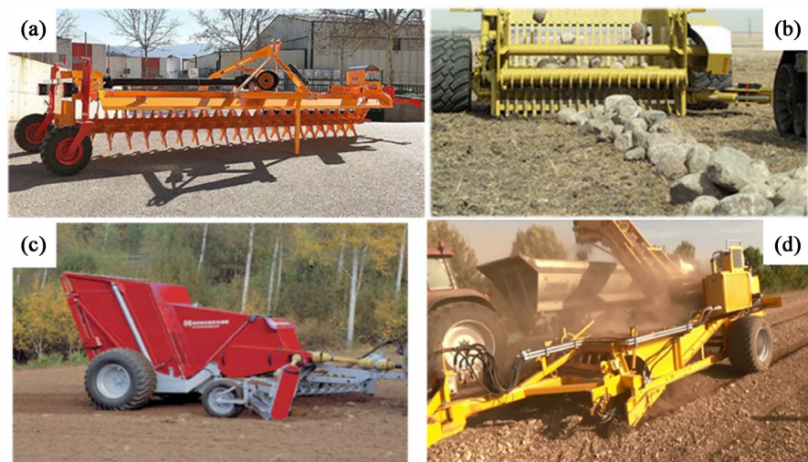
Figure 3. Samples of: (a) Stone windrower; (b) Stone picker; (c) Stone windrower & picker; (d) Stone collector with conveyor belt.
