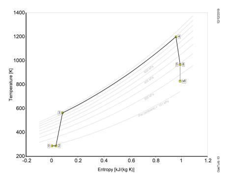
Figure 2. T-S diagram of the design point analysis without afterburner.
