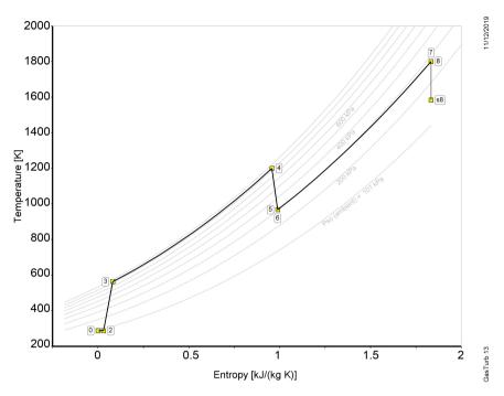
Figure 3. T-S diagram of the design point with afterburner.
