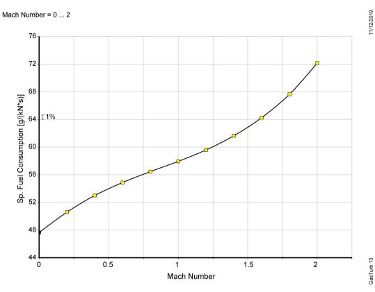
Figure 9. Specific fuel consumption against Ma at 10,000 m for Off-design performance.
