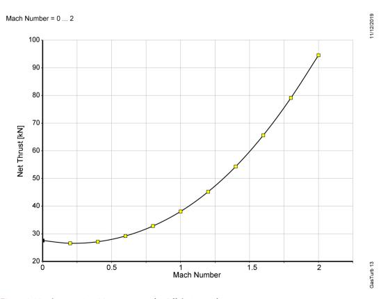
Figure 8. Net thrust against Ma at 10,000 m for Off-design performance.
