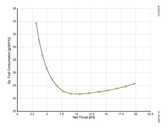
Figure 15. Engine operating line.
