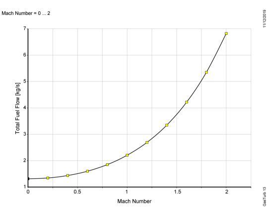
Figure 7. Fuel flow against at 10,000 m for Off-design performance.
