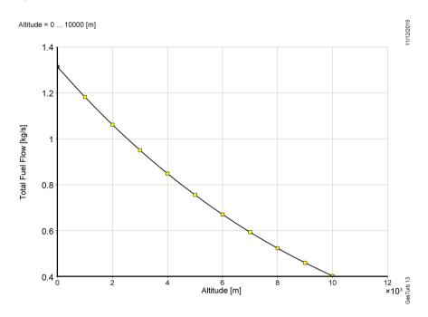
Figure 6. Fuel flow against altitude at Ma = 0.8 for off design performance.
