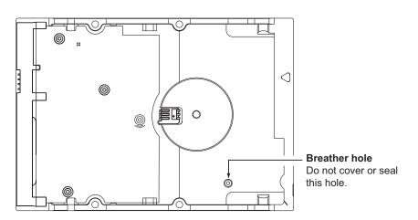
Figure 3 Breather filter hole location
