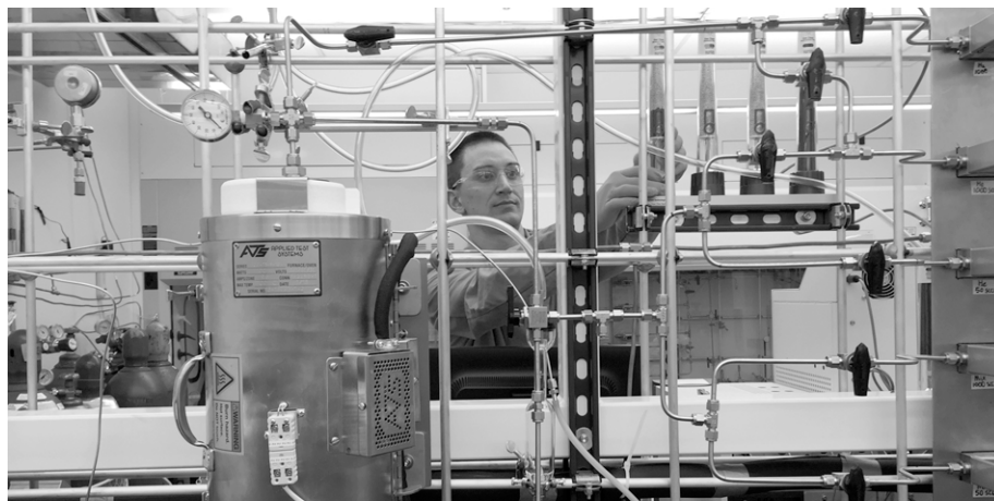
Chemical and biomolecular engineering assistant professor Dante A. Simonetti sets up a packed bed reactor.
