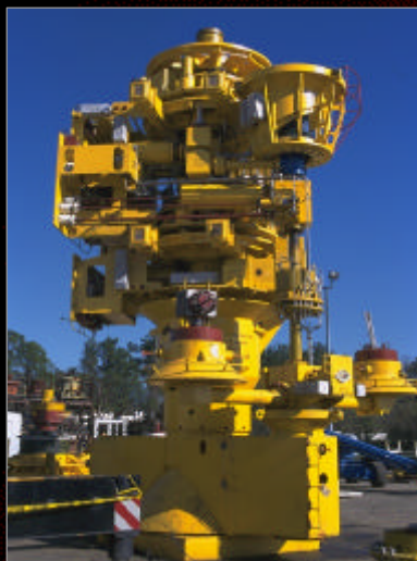
Subsea Tree with Controls
