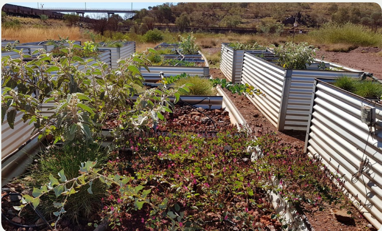
Raised vegetation beds installed at a field station in the Pilbara constructed to examine effects of inorganic amendments and plant community type on mine waste substrate properties and plant growth over a three-year period (Image: David Merritt).
