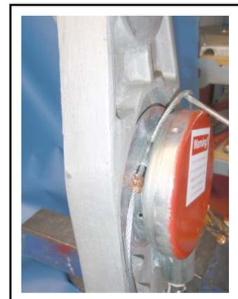
6. Using needle nose pliers, create slack in the cable by pulling the copper swage close to the drum.
