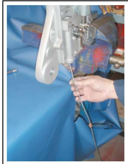
2. Once the tripline has passed through the trip block, bend the end of the tripline into a tight spiral using a pair of pliers.
