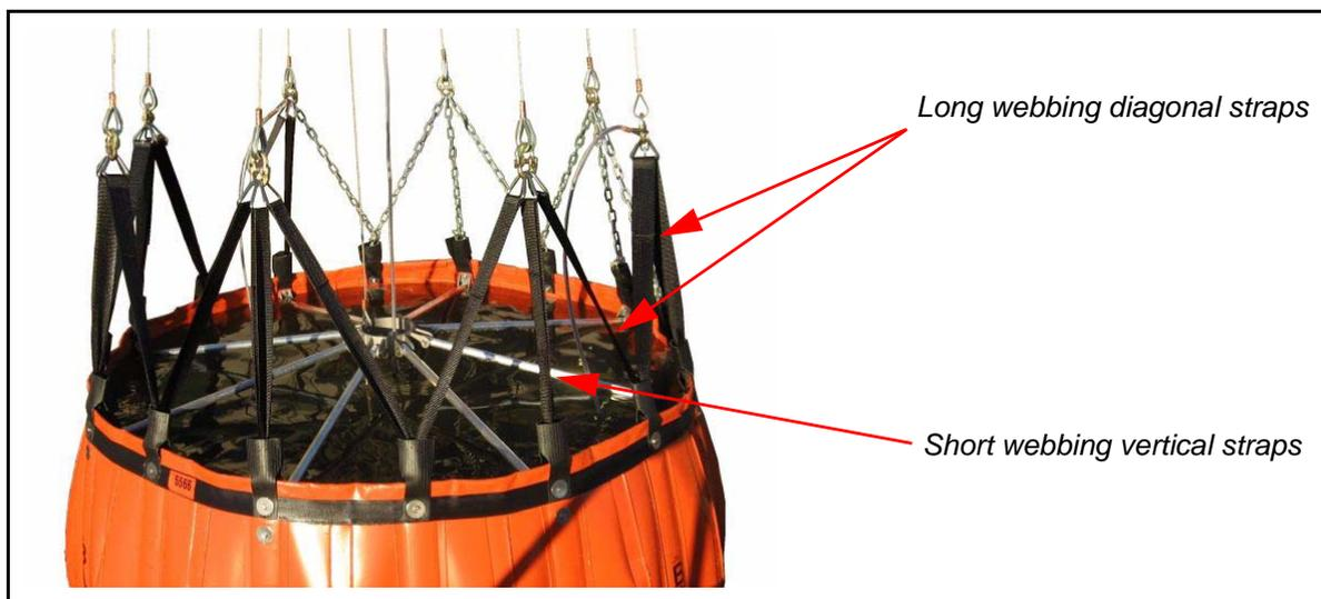
When replacing straps, do one set at a time to avoid confusion. Cut off the old straps from the shackle and un-tie them from the top of the bucket shell. Attach replacement straps as per the originals.
