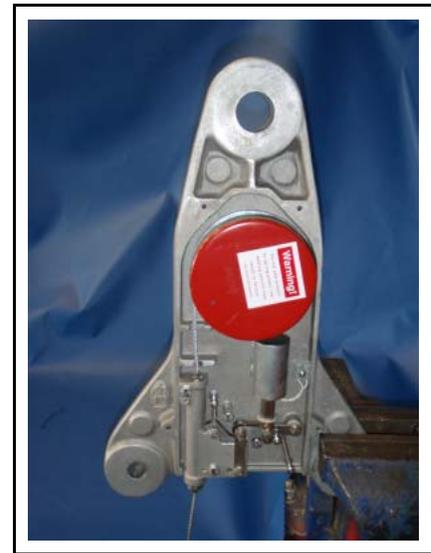
2. If the tripline is not broken above the trip block and the spring reel is functional, push the solenoid up locking the catch open with a bolt or pin and pull the tripline out to its full extent.
