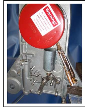
4. Stop spring reel when the openings are at the top.
