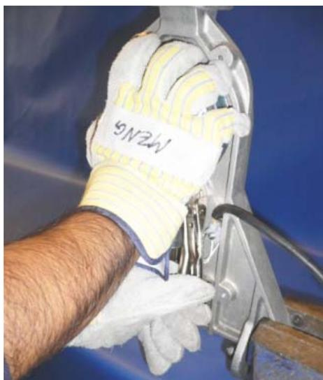
*Removing the locking device.*
