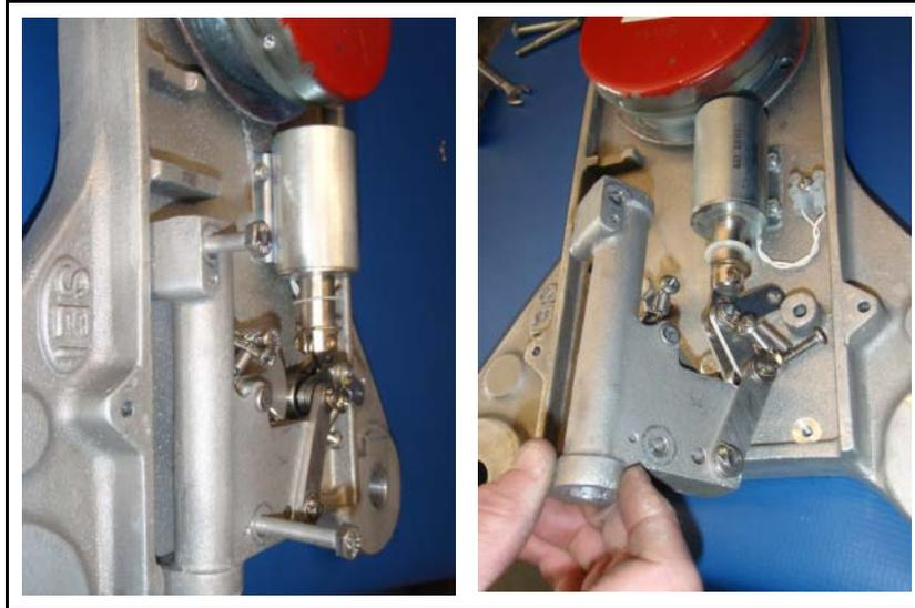
5. Remove the clevis pin, holding the catch in place. The catch can now be removed from the slot.
