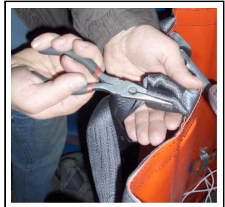
***Installing New M-Straps (Short)***
