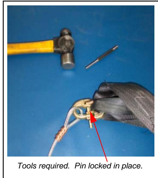
To remove the connecting link (connecting the suspension line to the M-strap) follow the procedures outlined below.
