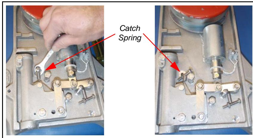
3. Disconnect the return spring mounting bolt and remove the clevis pin above the return spring mounting hole.
