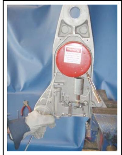
9. Wrap the vinyl covered cable back around the spring reel. Remove the temporary lock and, again, pull the cable out until the reel stops.
