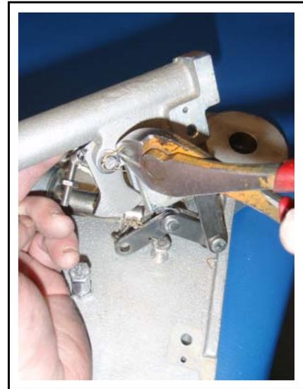
8. Remount the trip block, the spring link clevis pin and the return spring mounting bolt.
