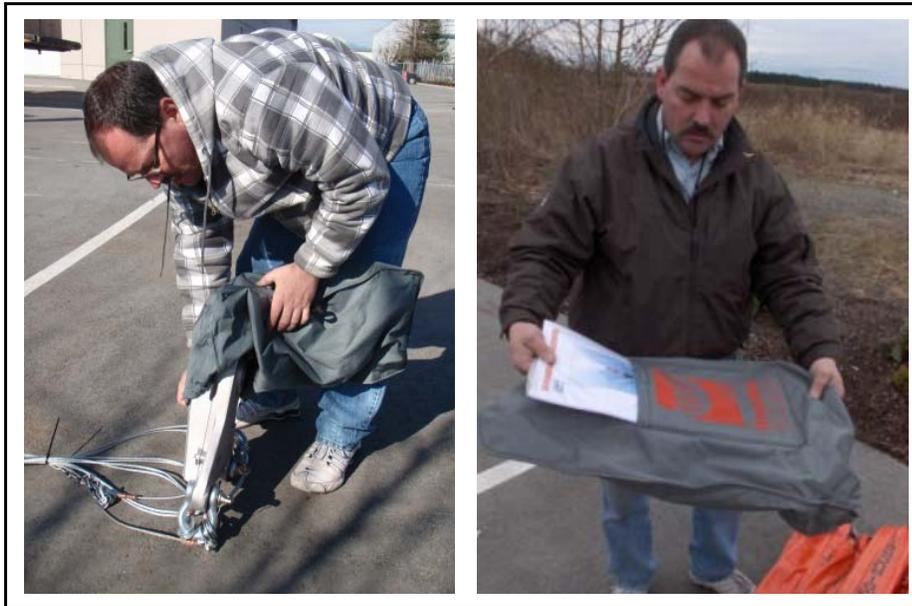
3. Gather the suspension lines into a coil and stow inside the bucket. Place the control head outside of the bucket to prevent the possibility of the lines tangling.
