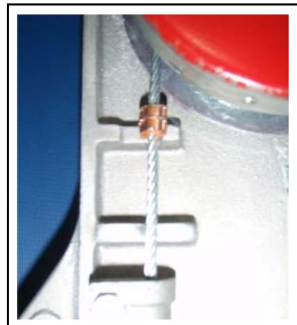
9. While holding the reel securely, release the temporary lock. Allow the cable to wind in gradually. Do not let the reel free-wheel. **Use gloves to protect your hands from injury.**
