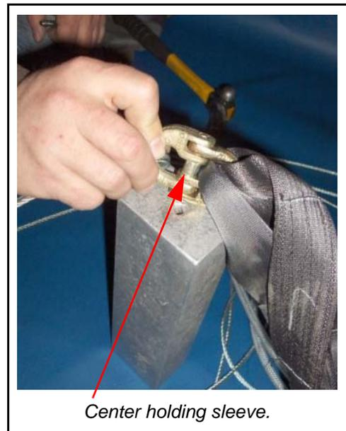
2. Place the connecting link with the pin located over the hole and using a 3/16" punch, drive pin through the center holding sleeve.
