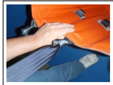
7. The M strap set should now look like this. The suspension line attaches to the top of each M-strap set.
