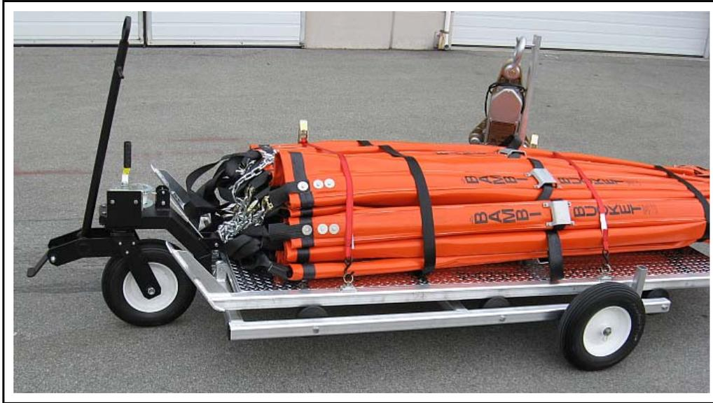
The rugged, lightweight two-piece Bambi Mobility Cart allows one person to move a bucket from one location to another. Easy to steer and brake, the three-wheeled cart comes equipped with tow-bar and foam-filled all-terrain 16" tires. Roll on, winch and go!
