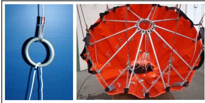
4. Thread the purse lines, alternating from one side of the valve to the other.
