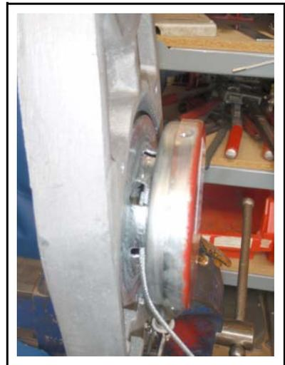
10. Back the spring reel off until the three holes are positioned at the top (approx. one full turn) and secure the reel.
