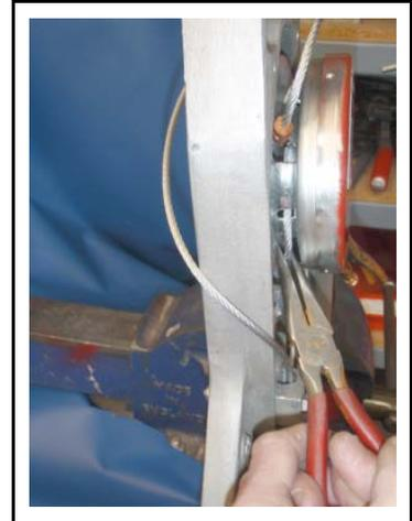
7. Use a small stiff wire through the hole in the spring reel drum to remove the end of the tripline from the locking finger.
