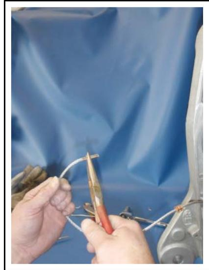
3. Insert the end of the tripline through the large center hole of the drum. Fish the tripline out through the small hole to the right of the center hole using a flat screw driver. Guide the end of the swage block out through the hole.
