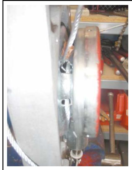
6. Pull the line up and over the finger and into the slot between the finger and the drum. To assist in this step:
