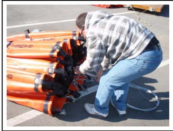
4. Place the head and Firesock on top of the bucket. Using the two straps supplied, strap the bucket to secure.
