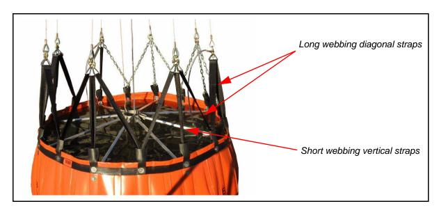
When replacing straps, do one set at a time to avoid confusion. Cut off the old straps from the shackle and un-tie them from the top of the bucket shell. Attach replacement straps as per the originals.
