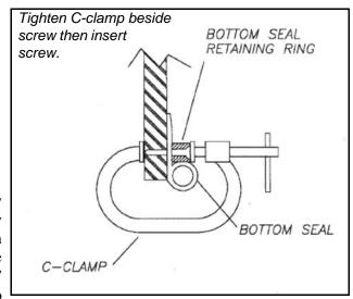
For the 27" aluminium valve body, all procedures are the same as above except 10-24 bolts and nuts are used with the bolt being inserted from inside the tube and the nut on the outside of the retaining ring.
