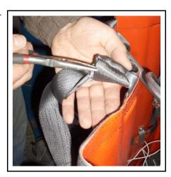
2. Fully insert the pliers at the far left hand side of the top layer.
