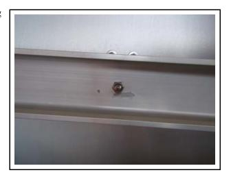
Remove the two socket head Allen screws securing the cable plate to the top slider tube.
