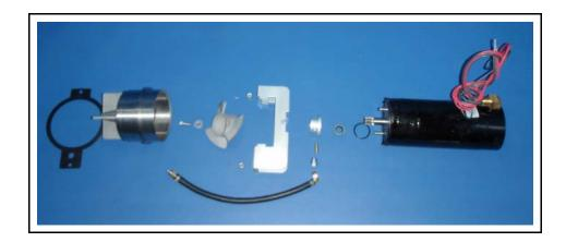
If disassembly of the pump progresses to the point that the seal cup is removed, it is recommended that the secondary seal and base o-ring be replaced. New seals and o-rings are available from SEI Industries.
