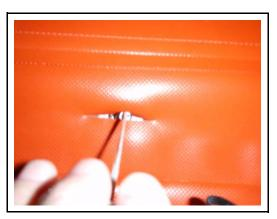
4. Place the top of the clamp over the bolt.
