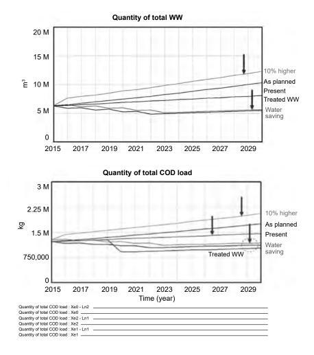
Figure 13.12. Changes in wastewater (WW) quantity and COD load under the six scenarios in the study area's water drainage network from present to 2030
