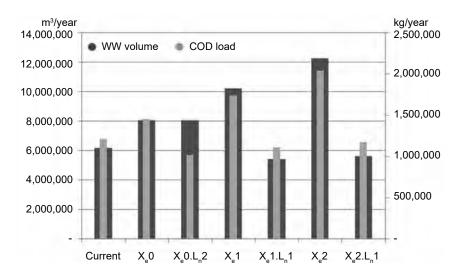
Figure 13.13. Changes in wastewater quantity and COD load under the six scenarios in the study area's water drainage network in 2030
