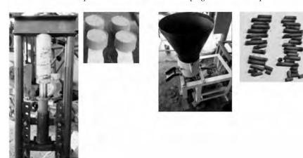
b. Cold densification system and briquettes
