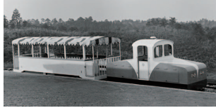
The Otogi Train, predecessor of today's Yamaguchi Line, used a battery-powered locomotive to pull its passenger carriages.
