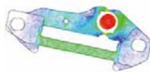
Simulation of the magnetic characteristics to the motor in analog quartz motor with lower power consumption
