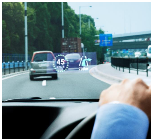
Wedge-shaped interlayer film for HUDs (improved HUD visibility)
