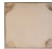
SUS445 Signs of corrosion just beginning to appear
