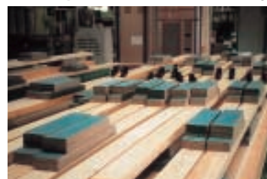
Cut-offs of exterior walls are used as vibration control blocks. (Higashinohon Sekisui Industry Co., Ltd.)
