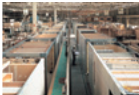
Sekisui Chemical's unit construction can perform over 80% of its house construction work at the plant, including the manufacturing of parts and materials and the assembling of each section of the house.
