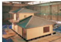
Earthquake-resistance testing using actual sized home
