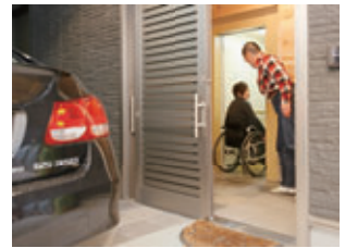
With the garage entryway sliding door divided by use, Mrs. Itoh can access the home from her car with a single wheelchair.
