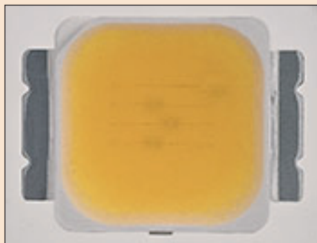
Cree's MX-3 LED, which has the same footprint and performance as the new high-voltage MX-3S LED.
