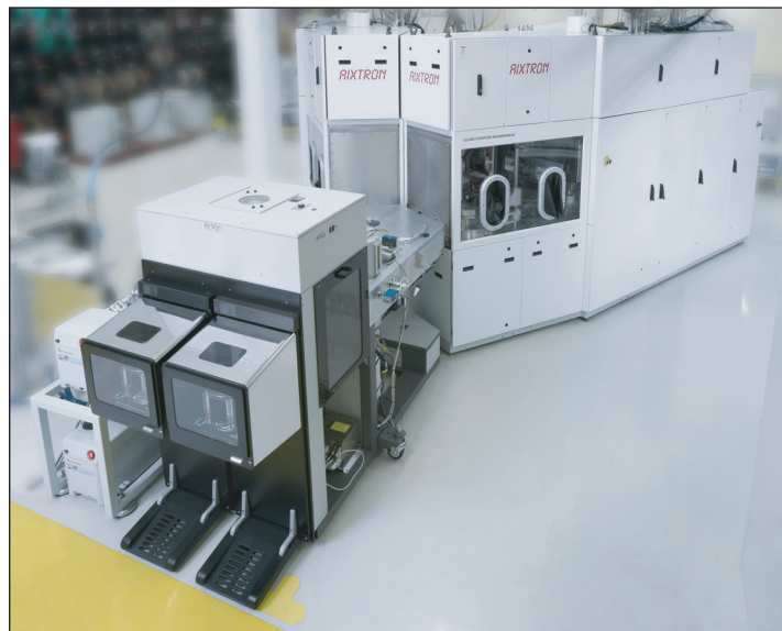
Figure 1. 300mm MOCVD cluster tool with two process modules for III-V on silicon processes.
