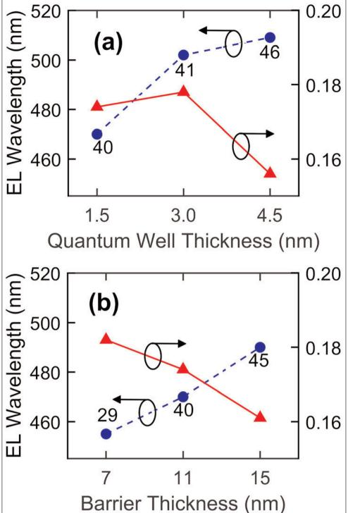
Figure 2. Electroluminescence wavelength and light output power versus (a) quantum well thickness with 11nm wide barriers and (b) barrier thickness with 1.5nm wide quantum wells. Wavelength points labeled with FWHM in nanometers.
