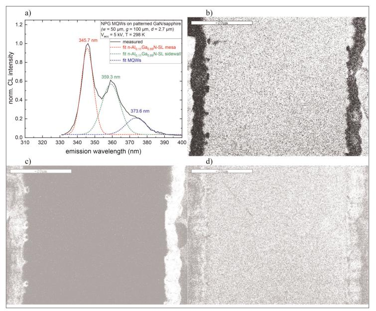
Figure 2. (a) CL spectra at room temperature of NPG MQW heterostructure and monochromatic CL maps at (b) 345.7, (c) 359.3 and (d) 373.6nm.
