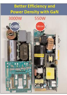
3000W GaN power supply versus 550W silicon power supply (Xuzhou GSR Semiconductor Co Ltd).
