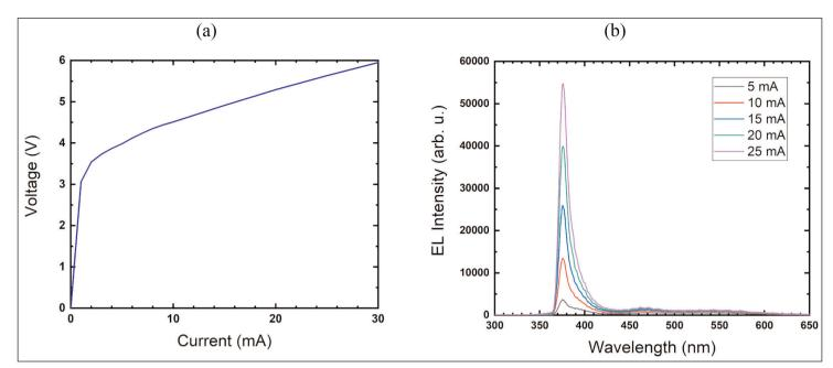
Figure 3. (a) Voltage-current plot and (b) 300K injection-current-dependent EL spectra of edge emission of a 30µm wide NPG/GaN/sapphire laser diode stripe for various DC drive currents.
