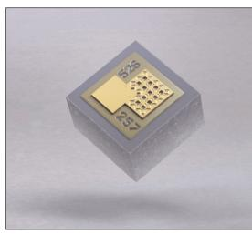
**New generation of 940nm-emitting VCSEL** has developed the patented array with 12 emitters for high optical output power to enhance the quality in proximity sensing and laser auto-focus applications. The
