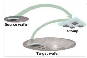
To facilitate the combination of these high-performance III-V optoelectronic materials in photonic devices, INSPIRE is developing wafer-scale micro-transfer printing technologies.
