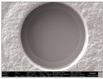
Polarization is locked by a surface grating etched directly into the GaAs. Polarization improves the illumination quality and resolution in demanding 3D illumination applications.
