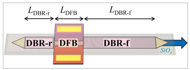
Figure 1. Longitudinal laser design for photon-photon resonance.
