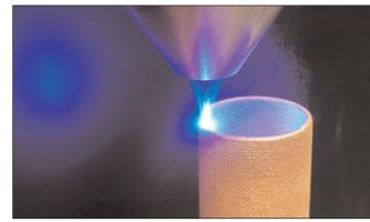
infrared radiation, this spectral range is absorbed much better by non-ferrous metals such as copper and gold. Among other benefits, this allows the heat conduction welding of copper components close to the surface, along with more energy-efficient and climatefriendly processes.
