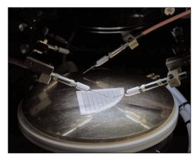
A transistor wafer undergoing testing on a probe station. Credit: Kate Myers/Penn State, Kelby Hochreither/Penn State.
