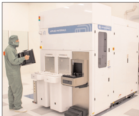
Applied Materials' eBeam metrology equipment in the cleanroom at Fraunhofer IPMS.
