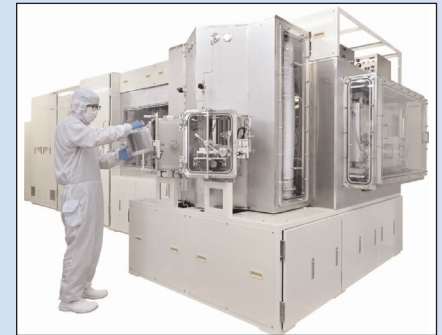
p48 Taiyo Nippon Sanso's new UR26K-CCD MOCVD system for the mass production of gallium nitride.
