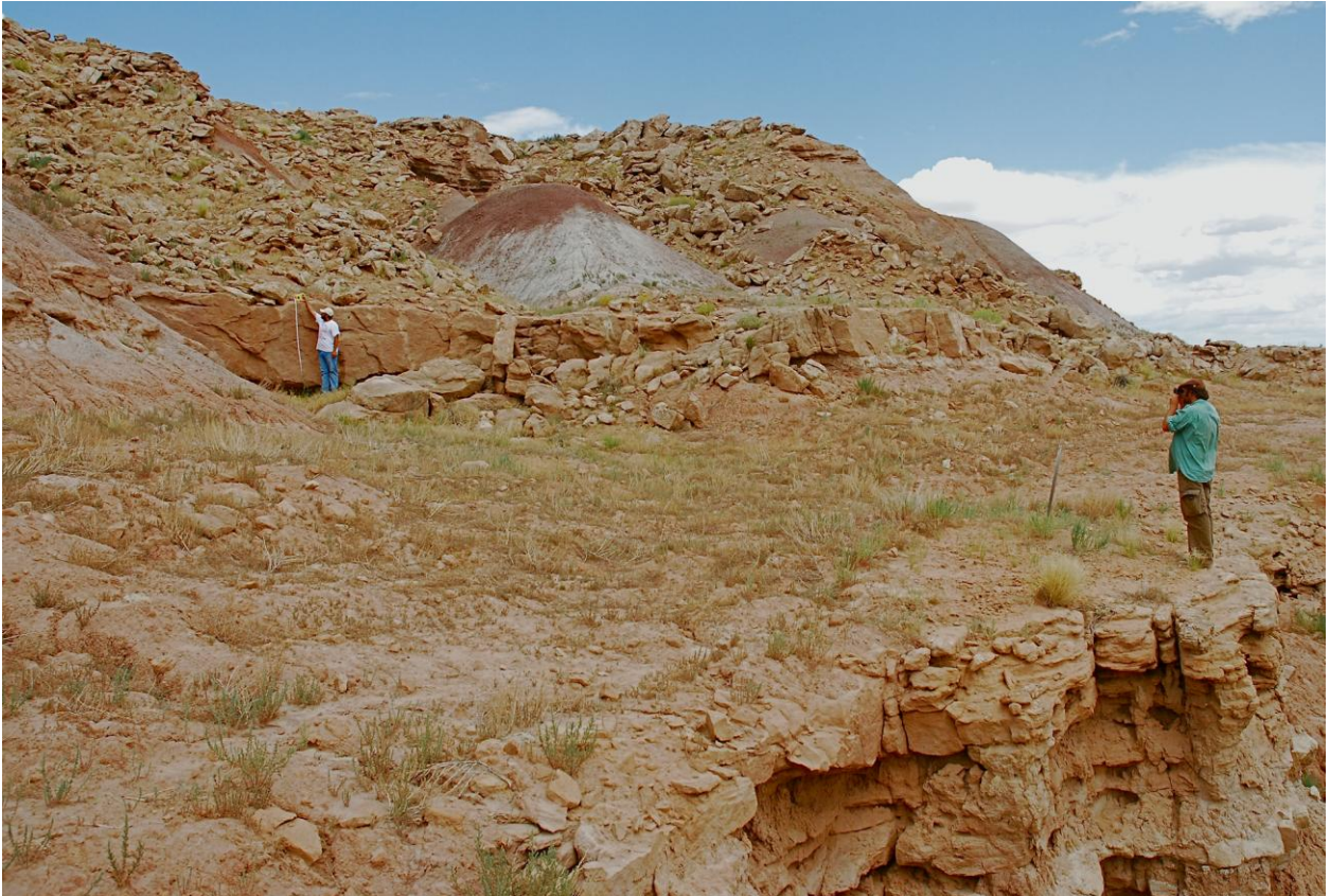
Figure 1. Mika and Burnes use a brunton compass and 50-meter tape to measure a Duchesne River Formation channel sand below the uppermost Uinta C outcrop on the west end of Deadman Bench.
