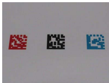
Figure 20 – Data Matrix Codes Printed in Color or on Colored Backgrounds
