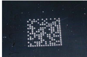
Figure 18 – Directly Marked Dot Matrix Code Characterized by Outstanding Separation Distance between Adjacent Code Elements
