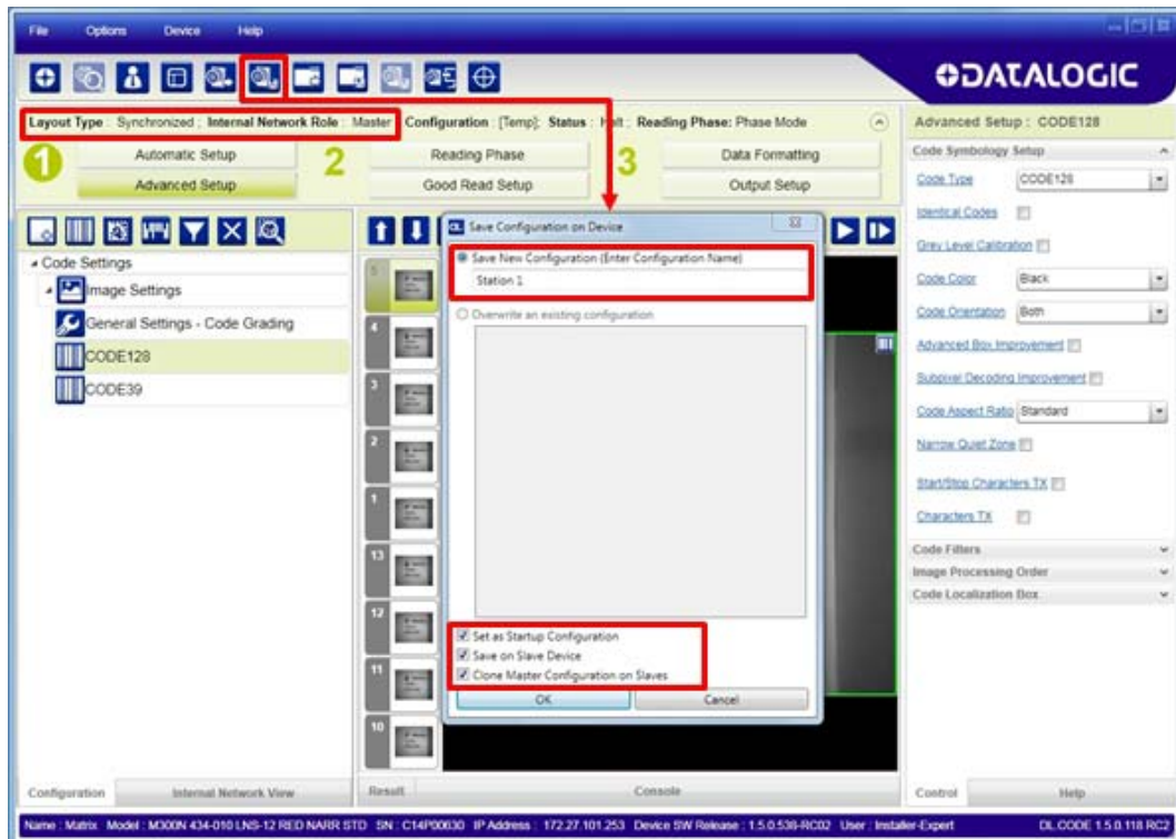
Figure 81 – Saving Synchronized Phase Mode Configuration to Master
