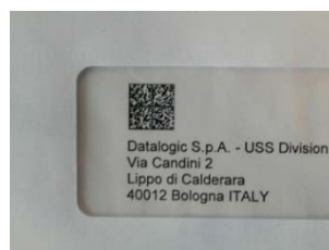
Figure 12 – Address Coded in Data Matrix Symbology for Automated Mail Processing
