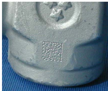
Figure 16 – Dot Matrix Code Directly Marked on Metal Surface by Using Dot Peening Technology
