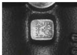
Dot Peening On Scratched Surface
