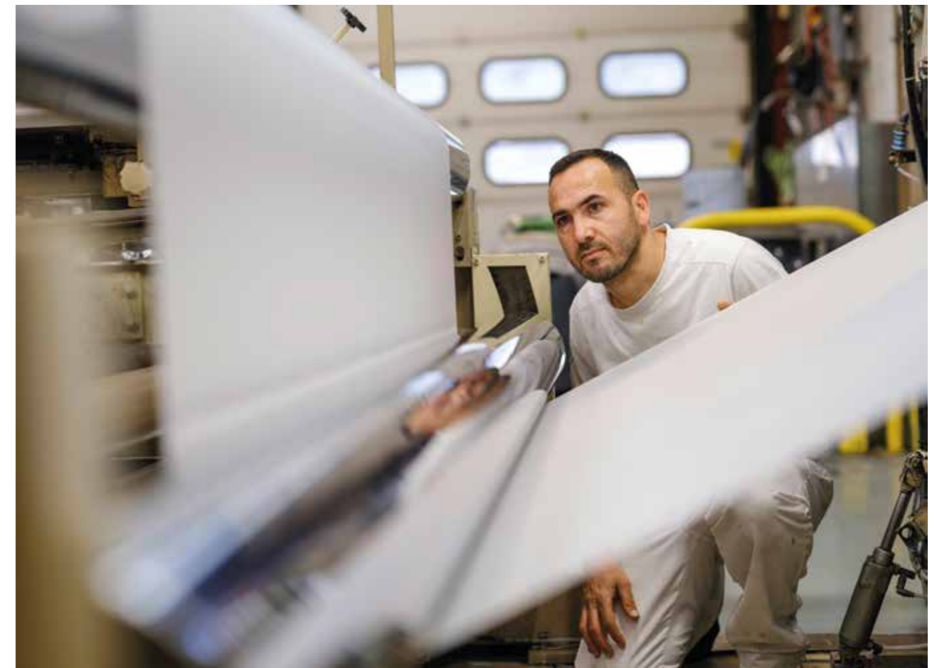
Surface checking of membrane rolls ■ La Tour-du-Pin
