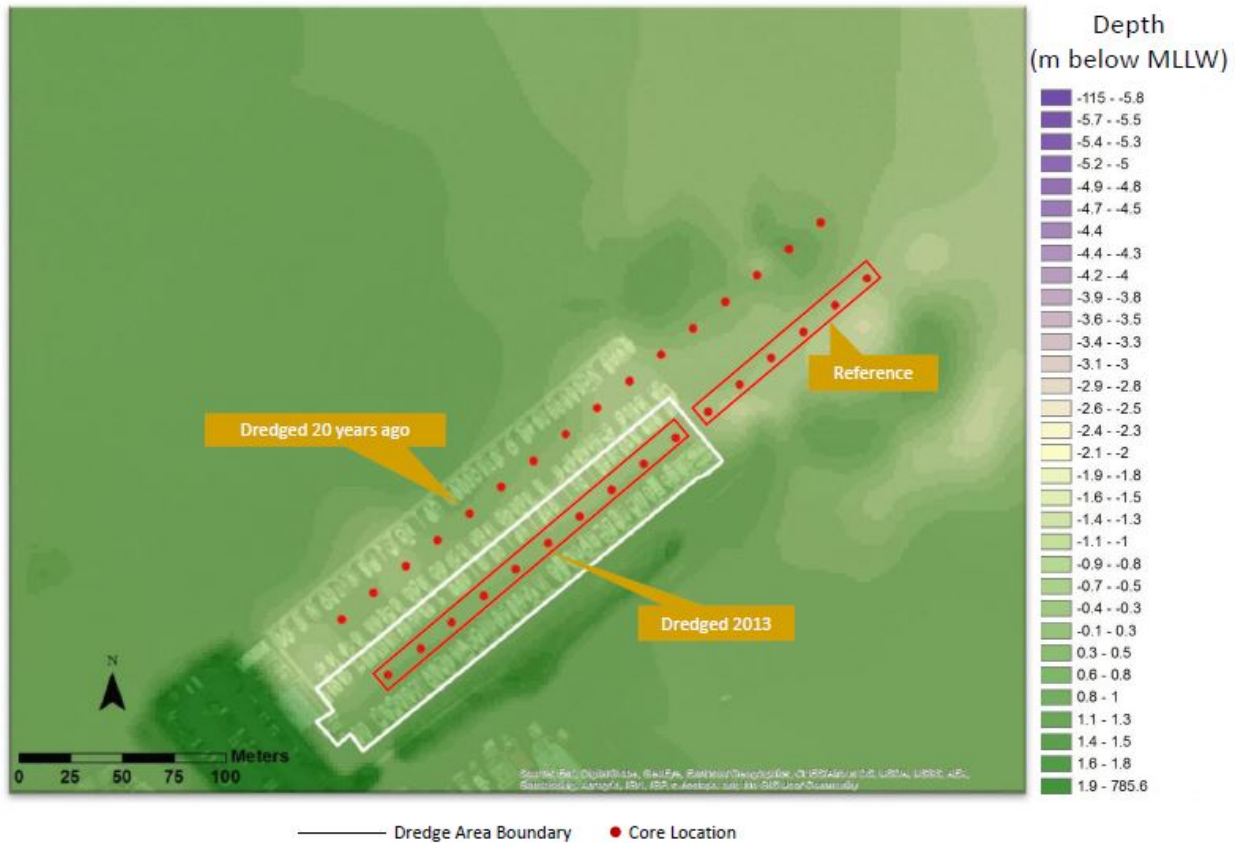
Figure 8. Richardson Bay Marina study site composed of marina docks and undredged reference area northeast of marina. Sampled as part of pilot and full study. White outlined area dredged to 10.5 ft MLLW in 2013. Site contains one transect of 10 core locations taken in area between docks that was dredged to 10.5 ft MLLW in 2013, another transect of 10 core locations in area between docks that was dredged in 1994. Two reference transects of six core locations each extend from the marina.
