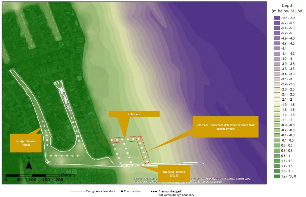
Figure 6. Paradise Cay HOA study site composed of residential docks and berths in western SFB. Sampled as part of pilot and full study. White outlined area dredged to 8 ft MLLW in 2014. Site contains 24 core locations in dredged area, 21 undredged reference core locations; three transects of six core locations in dredged marina, one transect of six core locations in dredged entrance channel, one reference transect of six core locations with three transects of five core locations extending from reference transect to dredged entrance channel transect.
