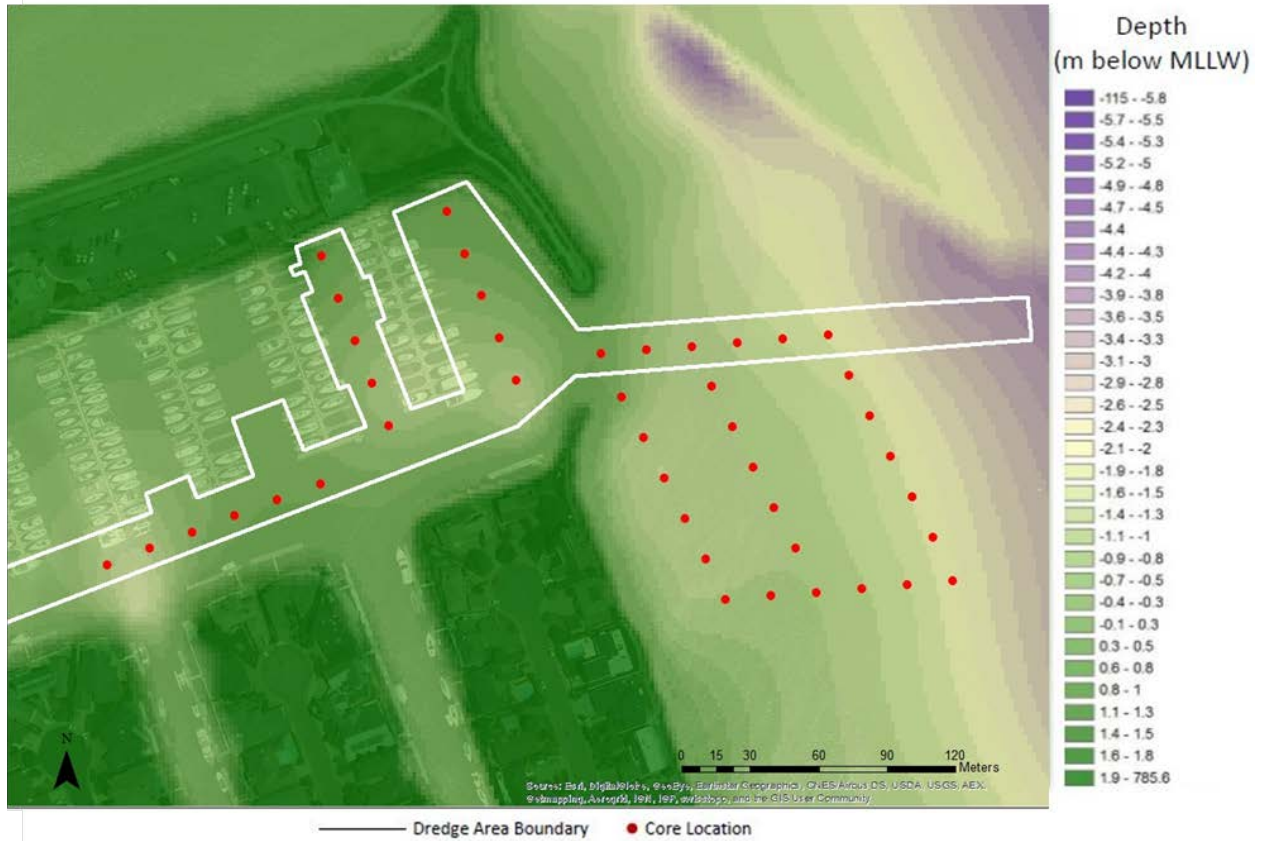
Figure 18. Paradise Cay Yacht Harbor study site composed of marina and entrance channel in western SFB. Sampled as part of full study. White outlined area dredged to 10 ft MLLW in 2015. Site contains 22 core locations in dredged area, 21 undredged reference core locations; three transects of five to six core locations in dredged marina, one transect of six core locations in dredged entrance channel, one reference transect of six core locations with three transects of five core locations extending from reference transect to dredged entrance channel transect.
