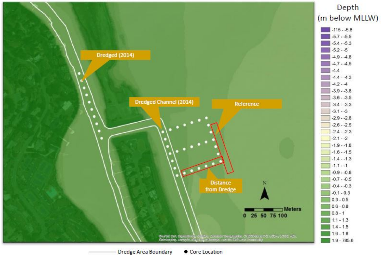
Figure 7. Strawberry Channel study site composed of residential docks and berths in dredged channel through residential area and Aramburu Island in Richardson Bay. Sampled as part of pilot and full study. White outlined area dredged to 7 ft MLLW in 2014. Site contains 10 core locations in dredged area, 12 undredged reference core locations; one transect of ten core locations and one transect of seven core locations in dredged marina/channel, one reference transect of seven core locations with three transects of five core locations extending from reference transect to dredged entrance channel transect.
