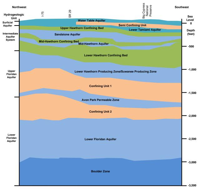
Generalized hydrogeologic cross-section of the LWC Planning Area (section extends from northwest Lee County through southeast Collier County).
