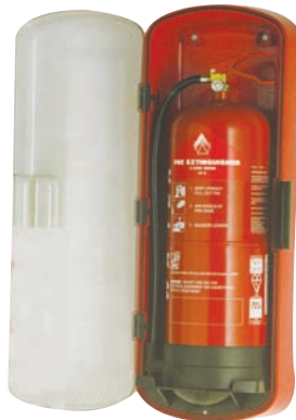
SINGLE FIRE EXTINGUISHER CABINET PN: TS101 • Storage of 9kg fire extinguisher • Dimensions: 762x282x211 • Aperture: 730Hx235W • GRP 3-4mm nominal thickness (Glass Reinforced Plastic)
