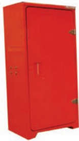
FIRE EXTINGUISHER CABINET PN: JB01 • Storage of 1 x 12kg or 12L fire extinguisher • Dimensions: 970x470x320 • Aperture: 760Hx275W • Weight 11 kgs • GRP 3-4mm nominal thickness (Glass Reinforced Plastic)
