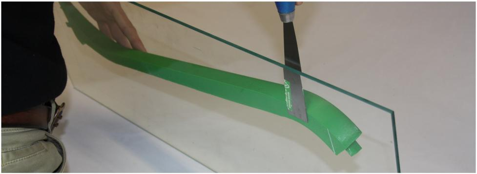
Remember that when printing is just completed, you may have the printing plate and certainly the extruder at high temperatures. The nozzle remains for several minutes at a temperature such as to cause a burn; check its temperature on lcd screen and absolutely avoid any contact with it if the indicated value is above 50 degrees. If in doubt, do not take out the glass until the temperature decreased to safe levels before you put your hands inside the print.
