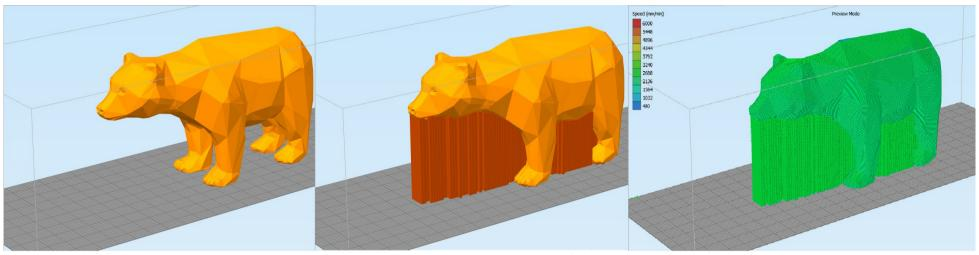
The support material are vertical structures generated -in this case – under the surfaces tilted over 45°.
