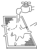
Fig. 12 —Cleaning filter with water or vacuum
