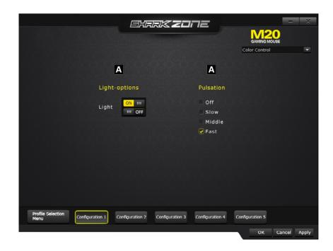
(A) Here the lighting of the mouse wheel can be turned on or off. Also, the speed of the pulsating lights (off, slow, medium, fast) can be adjusted and customized.
