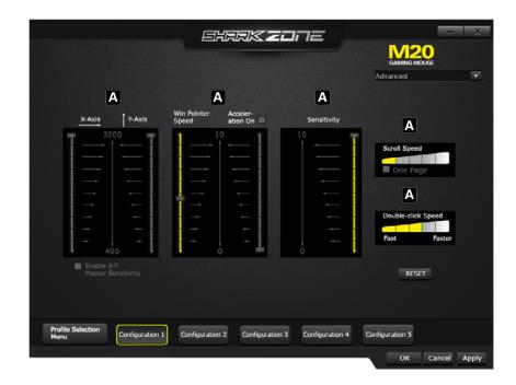
(A) In this field, the double-click, scroll speed, X-Y Master Sensitivity, Win Pointer Speed and Sensitivity can be adjusted.
