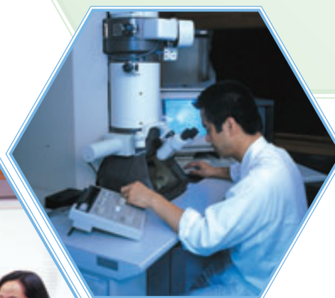
The JEOL-1220 transmission electron microscope allows Shionogi researchers to study the effects of diseases and candidate drugs on cells down to the nanolevel.
