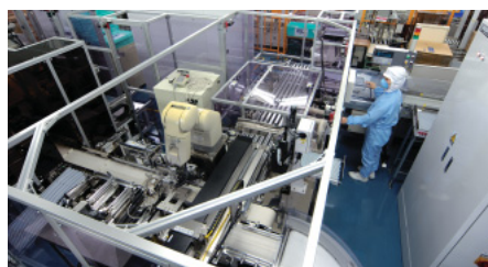
Robotic equipment seals cartons in a high-speed tablet and capsule filling and press-through packaging (PTP) line.
