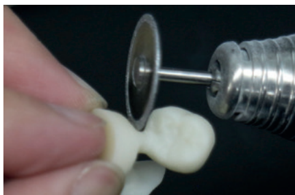
Use a fine diamond disk at low speed to cut the sprues
