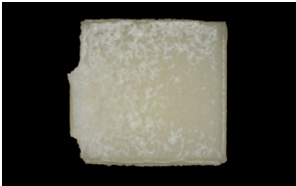
VINTAGE LD Press after glass bead blasting at 0.3 MPa (3 bar) pressure
