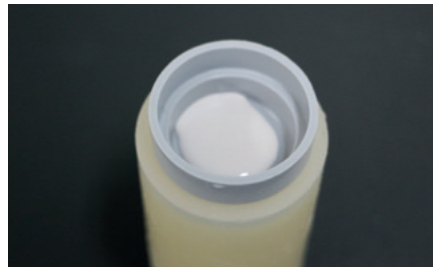
Place the ring cap on top of the ring to keep the top surface and bottom surface parallel.
