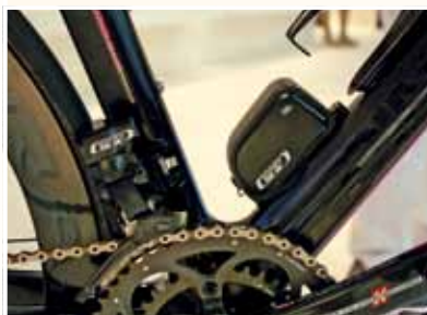
THE PINARELLO DOGMA, SPORTING THE LATEST VERSION OF CAMPAGNOLO'S SUPER RECORD ELECTRONIC GROUPSET.
