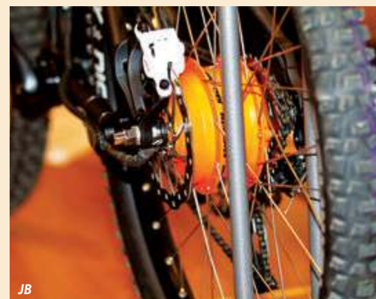
A close-up of Panasonic's new rear wheel hub motor, which will debut on a 650B off-road e-bike from KTM.
