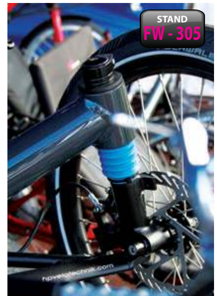
The full suspension system on the new Scorpion trike takes its inspiration from the car industry.
