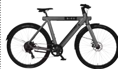
Bird A-Frame version with 250W Bafang rear motor and 346Wh/36V removable battery
