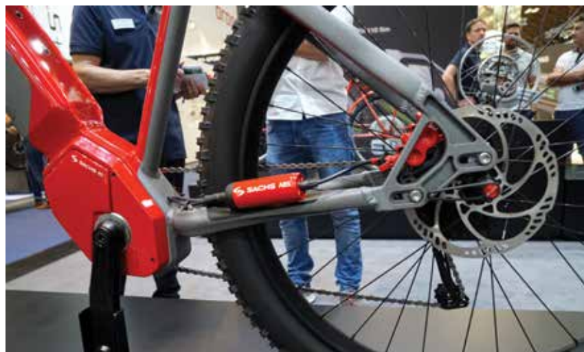
Brakeforce One/Sachs Micro Mobility ABS system
