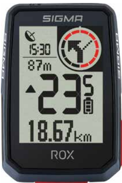
Even Sigma's low-end Rox 2.0 computers are equipped with GPS and turn-by-turn navigation
