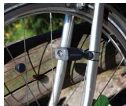
Reelight's Cio lights use magnetic induction to generate power
