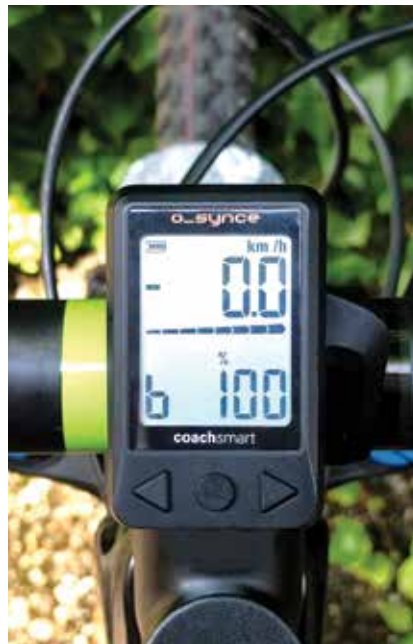
Coachsmart by O-synce: wide e-bike compatibility thanks to the ANT+ LEV connection
