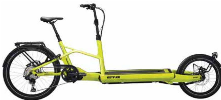
Kettler Cargoline series with Ackerman steering
