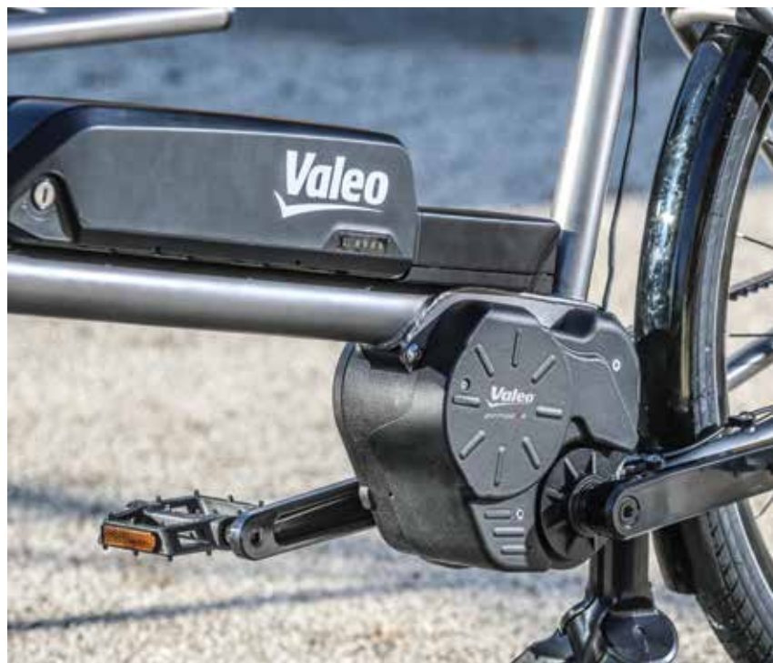
Valeo's Smart e-Bike motor with integrated adaptive automated shifting system
