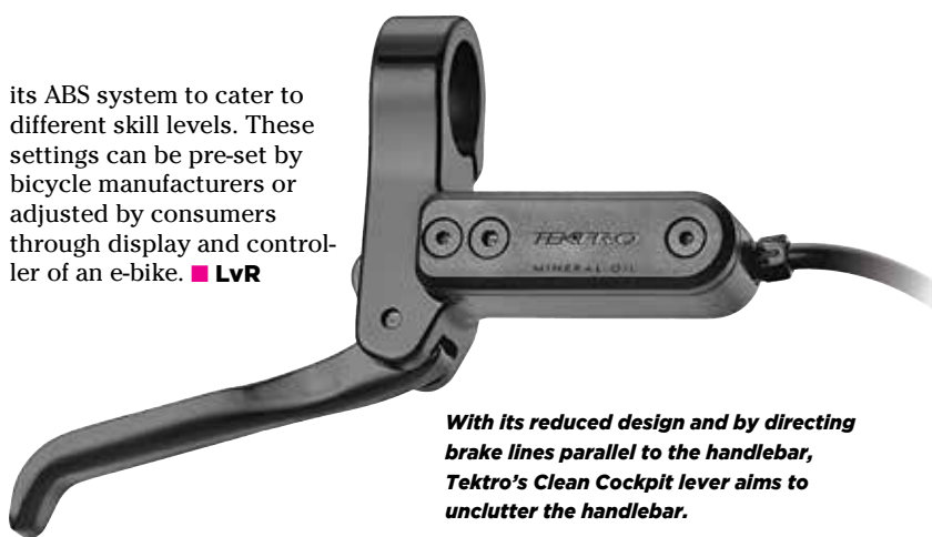
Tektro's and TRP's hydraulic disc brakes now also work with the second generation of Bosch eBike's ABS system.
