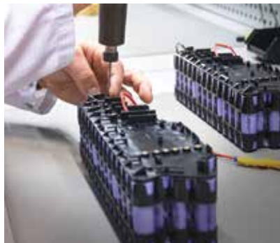
E-bike batteries are assembled from a sizable number of cells.
