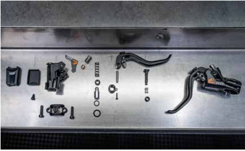
The parts that are needed to assemble a hydraulic disc brake lever at Magura
