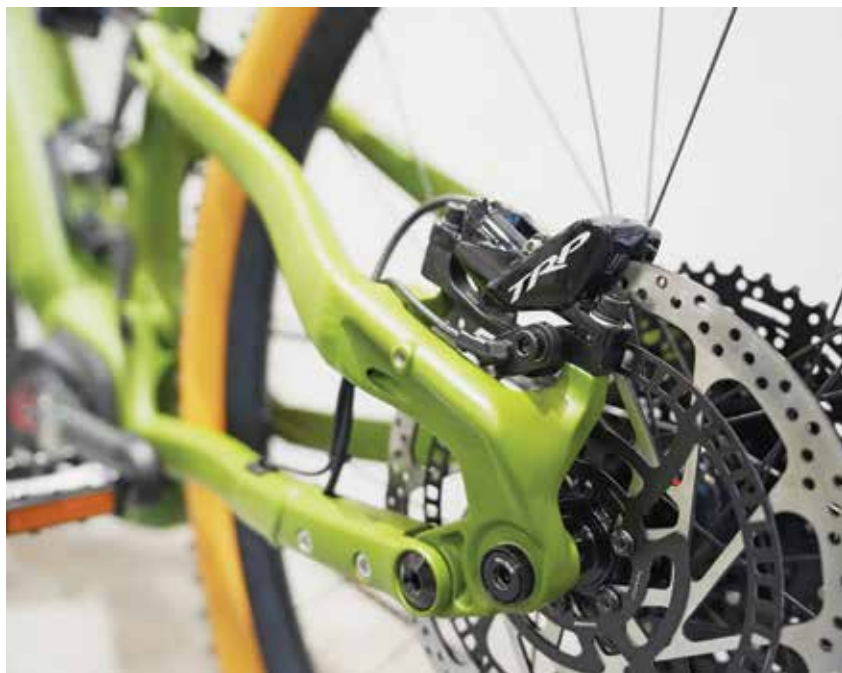
Tektro's and TRP's hydraulic disc brakes now also work with the second generation of Bosch eBike's ABS system.
