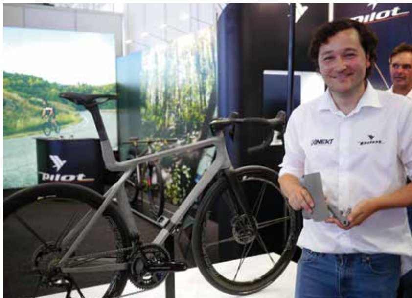
Tim Blankers with Pilot's 3D printed titanium Seiren road bike
