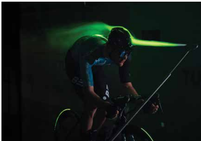
Agu's Transonic and Subsonic helmets are wind tunnel tested
