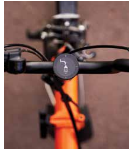
Keep it Simple is the motto of the Beeline Velo 2. The desired route is calculated via an app, and navigation works surprisingly well due to the clear track line and indicated path intersections.
