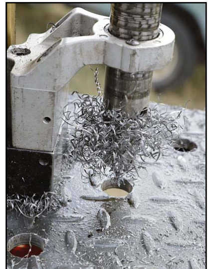
Above: It required 24mm holes to be drilled (with permission) using Ian's specialist drill.
