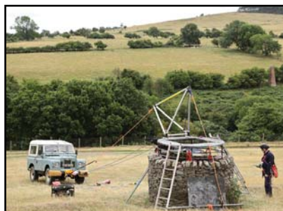
Left: Using a Land Rover belay the frame can then be used for hauling (or lowering) people in Sheep shaft.
