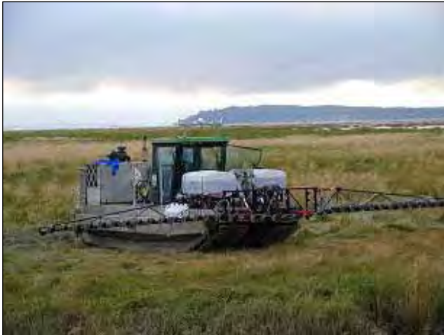
Fig. 6. Tracked amphibious machine with ground broadcast herbicide application equipment, Willapa Bay, Washington, USA.
