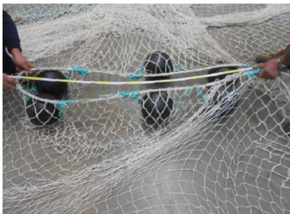
Figure XVI.1.4. Measurement of the headline at the bosom level. We measured 1.46 m, which multiplied by two is 2.92 m.
