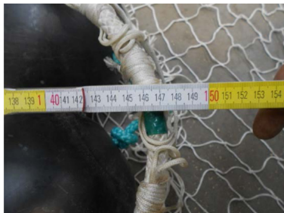
Figure XVI.1.4. Measurement of the headline at the bosom level. We measured 1.46 m, which multiplied by two is 2.92 m.
