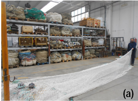
Figure XVI.1.9. Identification of the beginning and the end of each netting by looking at the transverse seams (a) and alignment of the transverse seams (b).
