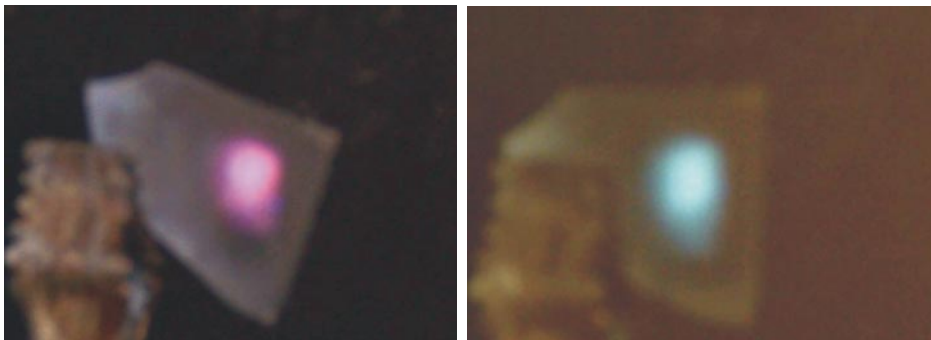
Figure 4. Photoluminescence recorded from the titania xerogel, doped with both Eu and Tb, confined in porous anodic alumina. A change in the emission colour with excitation wavelength is revealed: (a-left) red emission at \lambda_{ex}=300 nm; (b-right) green emission at \lambda_{ex}=365 nm.
