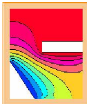
Fig. 2. A field of potentials in near-cathode areas of Spindt's cathode.
