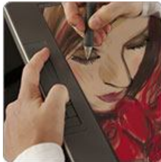
Fig.3. Capabilities of the ID Cintiq from Wacom, this display uses electromagnetic resonance principle to determine the coordinates of the contact point and the force-sensitive pen-tip to measure the applied force.
