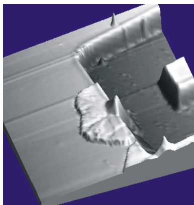
Figure 2. 3D AFM image of \text{SiO}_2 surface at borderline of p-n junction. 1, 2- amorphous \text{SiO}_2 over p-Si and n-Si respectively. K- microcrystals assemblage.
