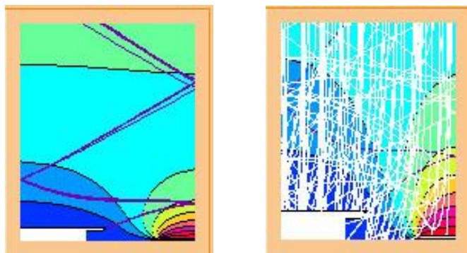
Fig. 6. (left) Potentials field and electron macro-particles movement trajectories in the “cathode-gate” area.
