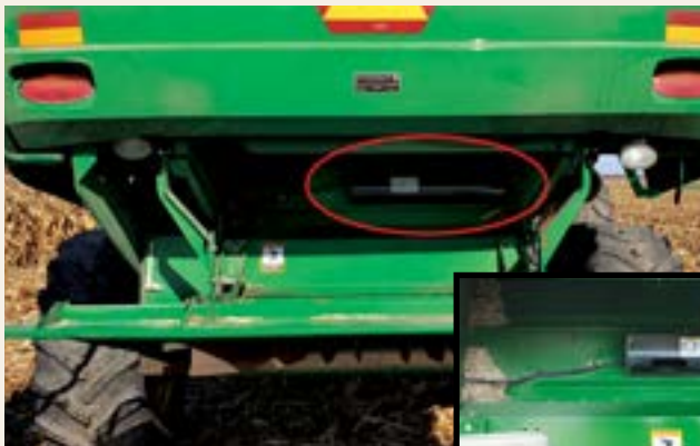
A tailboard, with Tailboard Trash Blower Tube, after a full season of harvesting soybeans.
