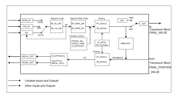
Figure 5-2 Function schematic of AO function block
