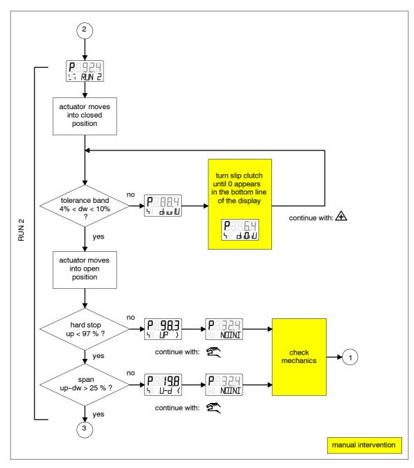
Figure 3-28 Automatic initialization, part 2 (for linear actuators)
