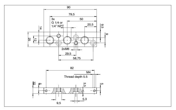
Figure 3-2 Dimensional drawing terminal strip for plastic housing
