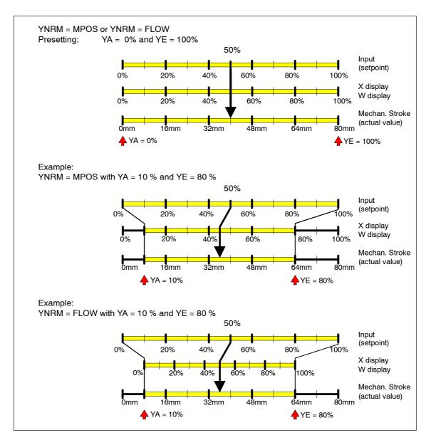
Figure 4-8 Dependence of the stroke on standardization and on YA and YE in the example of an 80 mm linear actuator
