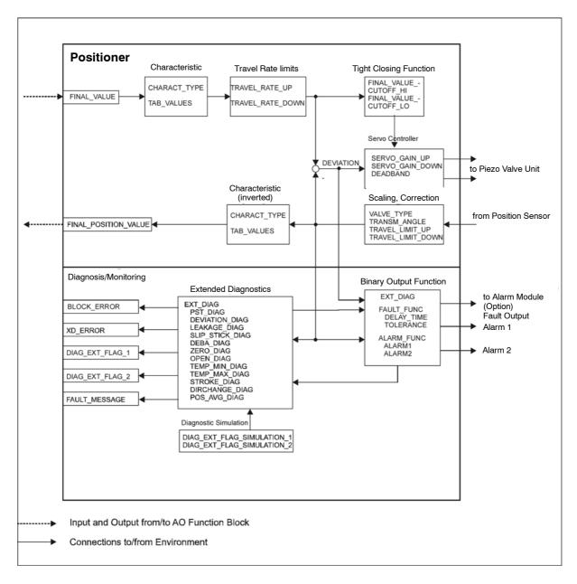
Figure 5-3 Function schematic of Analog Output transducer block
