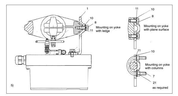
Figure 3-7 Assembly procedure (linear actuator) continued
