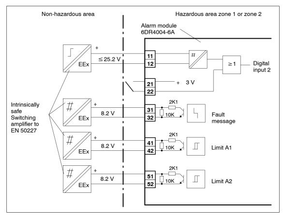
Figure 3-23 Alarm module 6DR4004-6A, EEx i
