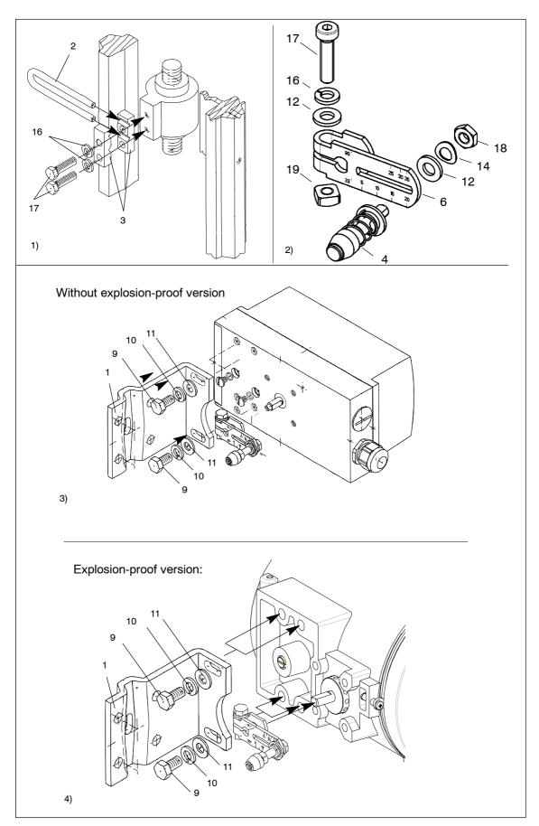
Figure 3-7 Assembly procedure (linear actuator)
