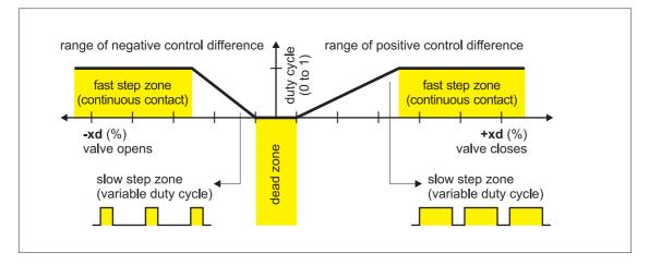
Figure 2-9 Method of operation five-point switch
