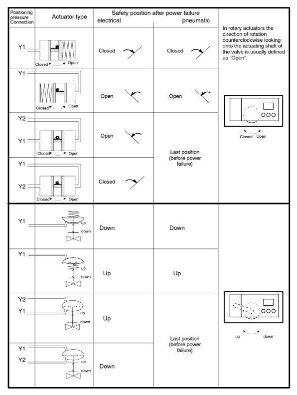
Figure 2-6 Pneumatic connection positioning
