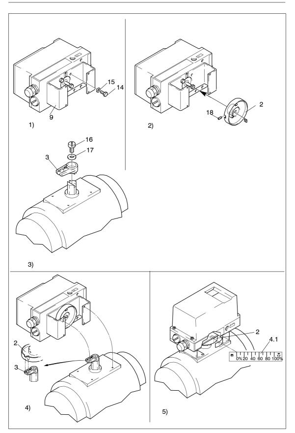
Figure 3-8 Assembly procedure (rotary actuator)
