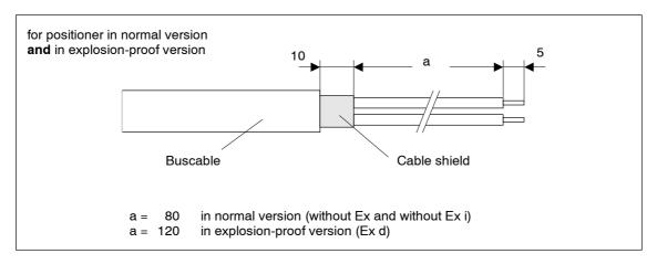
Figure 3-13 Preparation of bus cable
