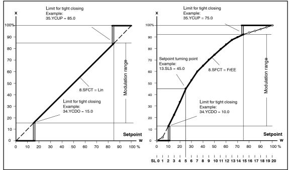
Figure 4-7 Setpoint characteristic, manipulated variable standardization and tight closing function
