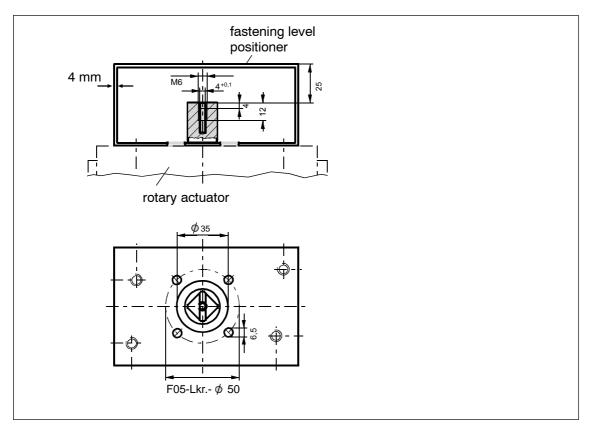
Figure 3-11 Attachment of rotary actuator, mounting console (scope of delivery actuator manufacturer), dimensions
