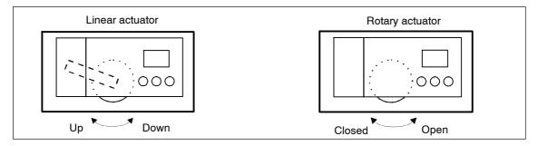
Figure 3-26 Direction of action of the actuators
