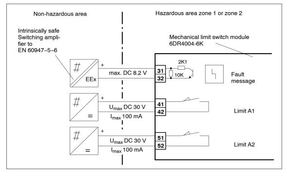
Figure 3-25 Mechnical limit switch module 6DR4004-6K, EEx i
