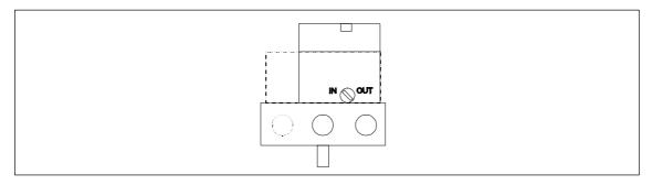
Figure 2-7 Purge air switch on the valve block, view of the positioner onto pneumatic connection side with cover open
