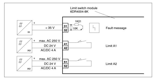
Figure 3-21 Mechanical limit switch module 6DR4004–8K, non Ex
