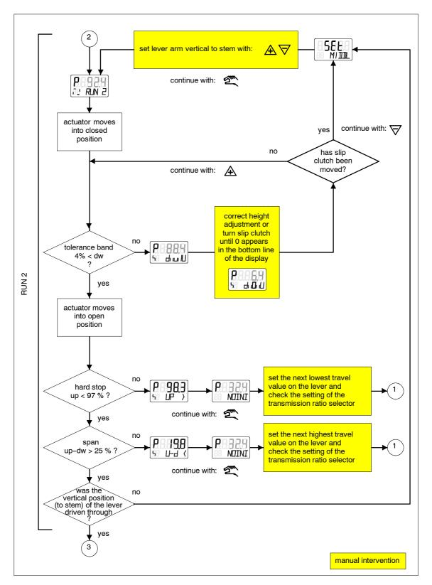
Figure 3-29 Automatic initialization part 2 (for rotary actuators)
